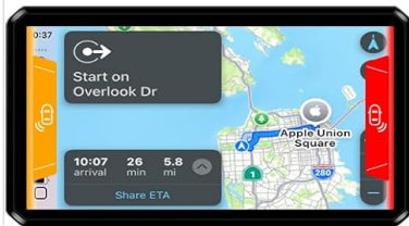
Figure 4.4: Visual representation of BSD (Blind Spot Detection), LCA (Lane Change Assist), and RCW (Rear-end Collision Warning) systems and their corresponding alerts on the display.
