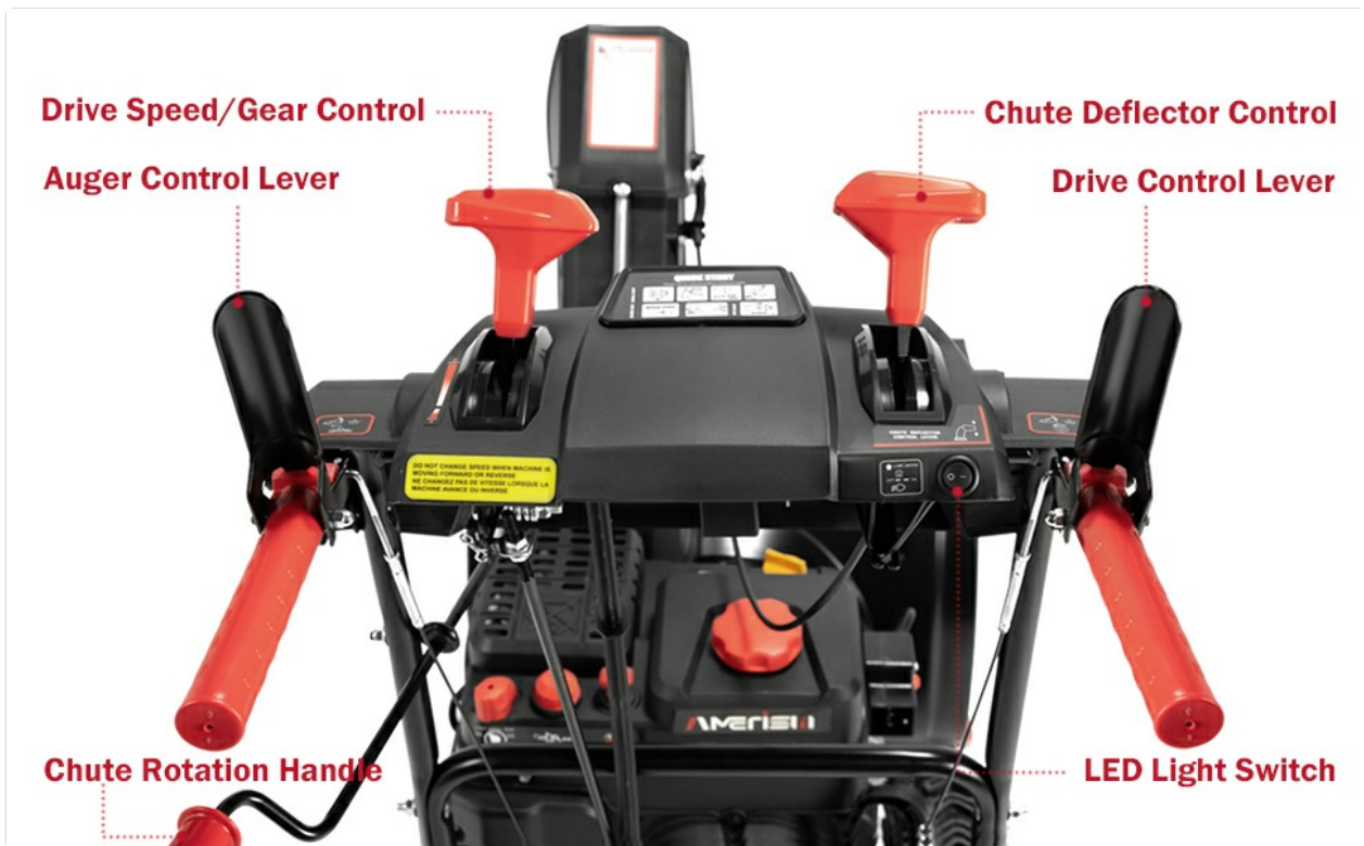
Image 4.2: Control panel layout with labeled functions.
