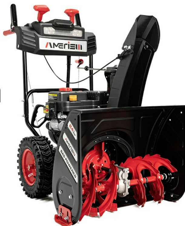
Image 1.1: Overview of the AMERISUN 24-Inch Two-Stage Gas Snow Blower.
