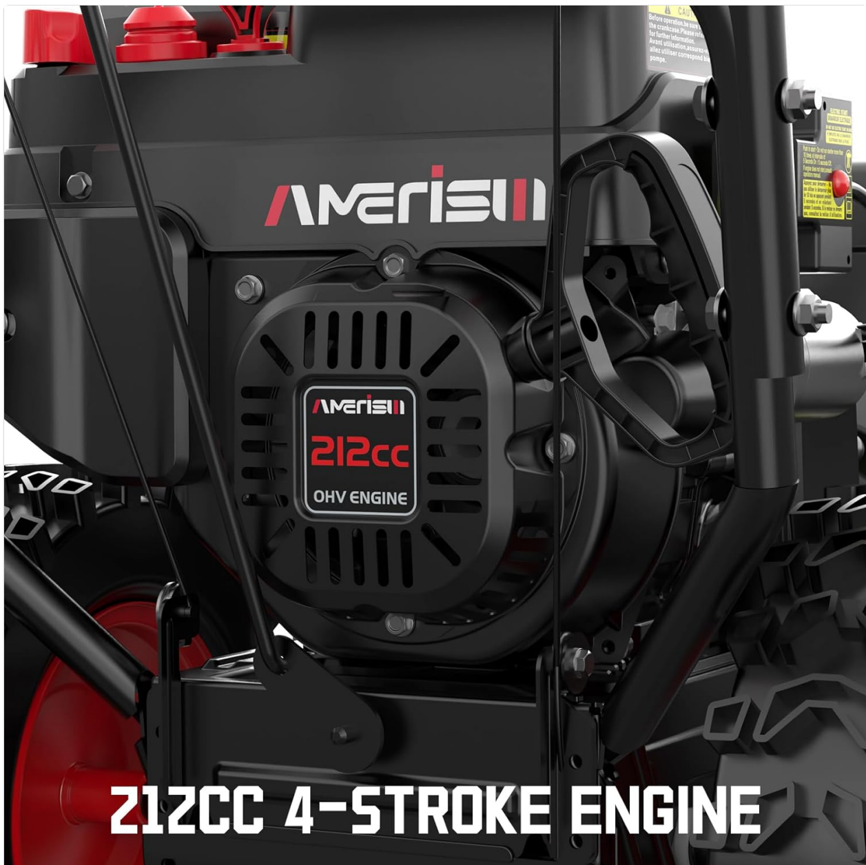
Image 4.1: The 212cc 4-cycle OHV engine.
