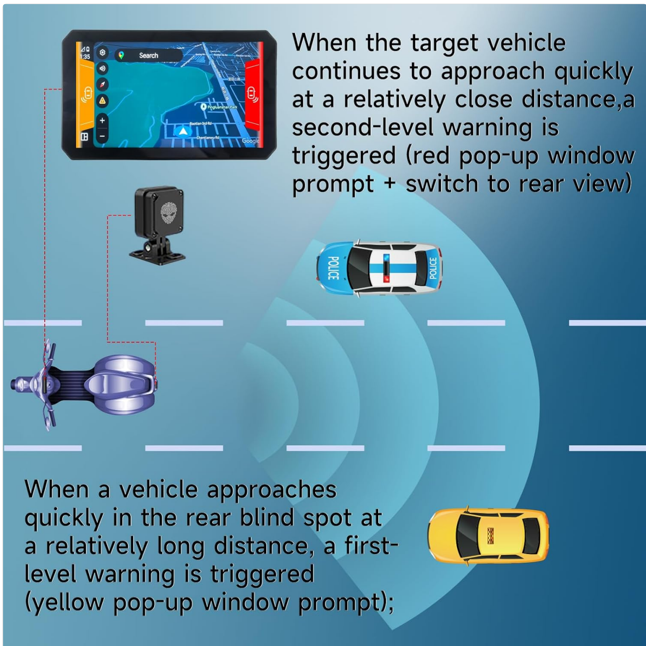
Figure 6.2: Blind Spot Warning Levels. This diagram illustrates the two levels of warnings: a first-level (yellow pop-up) for a vehicle approaching at a long distance in the rear blind spot, and a second-level (red pop-up with rear view switch) for a target vehicle approaching quickly at a close distance.
