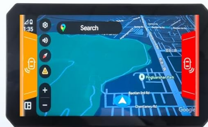
LCA Lane Change Assist Warning
