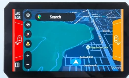
RCW Rear-end Collision Warning
