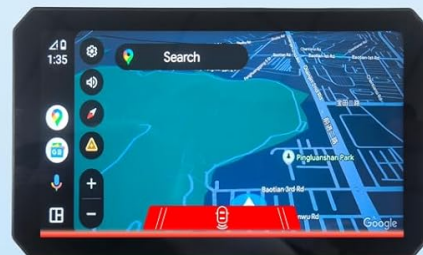
RCW Rear-end Collision Warning
