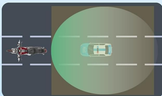
RCW Rear-end Collision Warning
