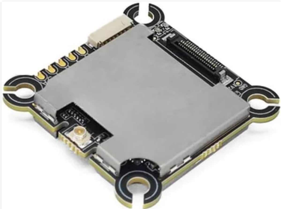
Figure 4: Angled view of the HDZero Whoop Lite VTX, highlighting the various connectors and mounting holes.
