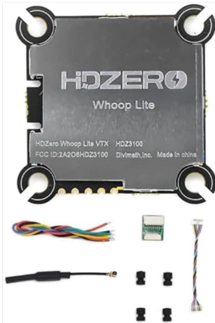
Figure 1: HDZero Whoop Lite VTX with its complete package contents, including the VTX module, connecting wires, dipole antenna, hardware, dampers, and zip ties.
