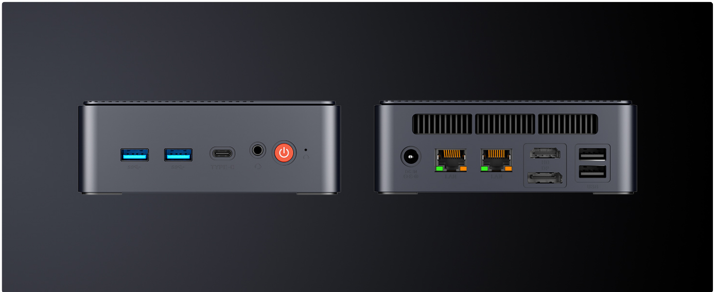
Image 3.2: Clear view of the front and rear connectivity options on the AWOW Mini PC AK11.
