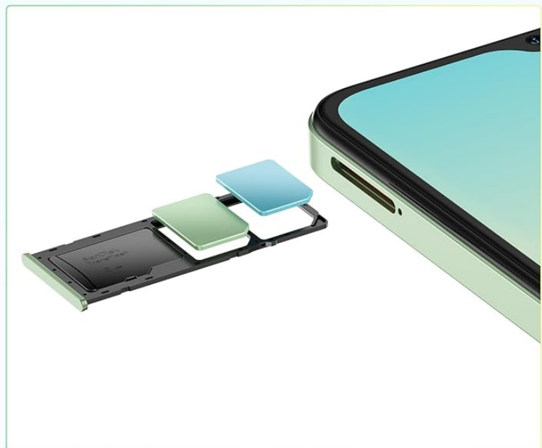
Figure 2.1: SIM and MicroSD Card Installation
