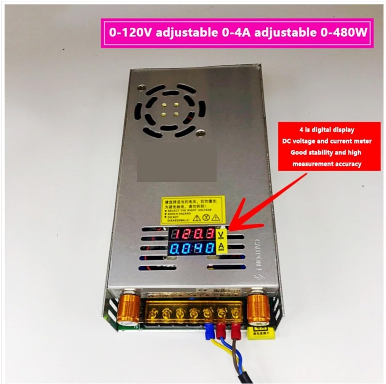
Figure 5.2: The digital display provides real-time monitoring of output voltage and current.
