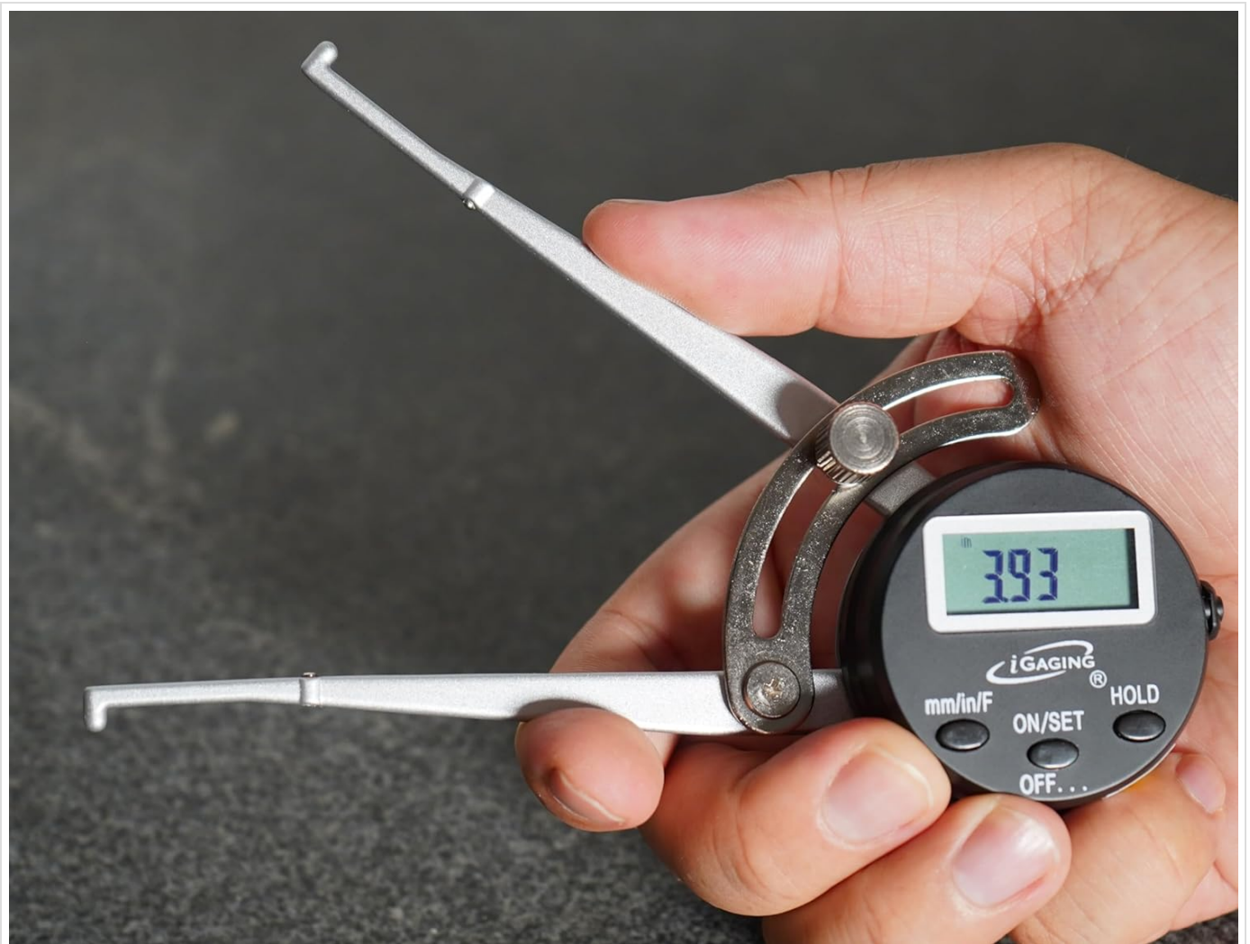
Figure 2: Proper technique for holding and using the digital inside caliper for measurement.
