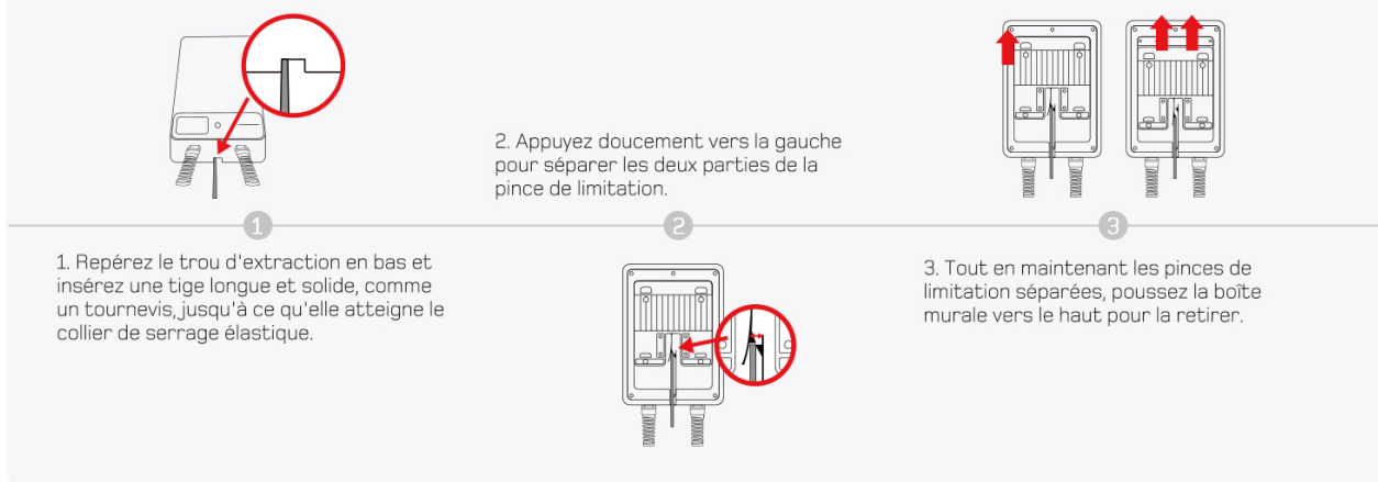
Image 4.1 : Wall mounting instructions for the dé Wallbox EV Charger.
