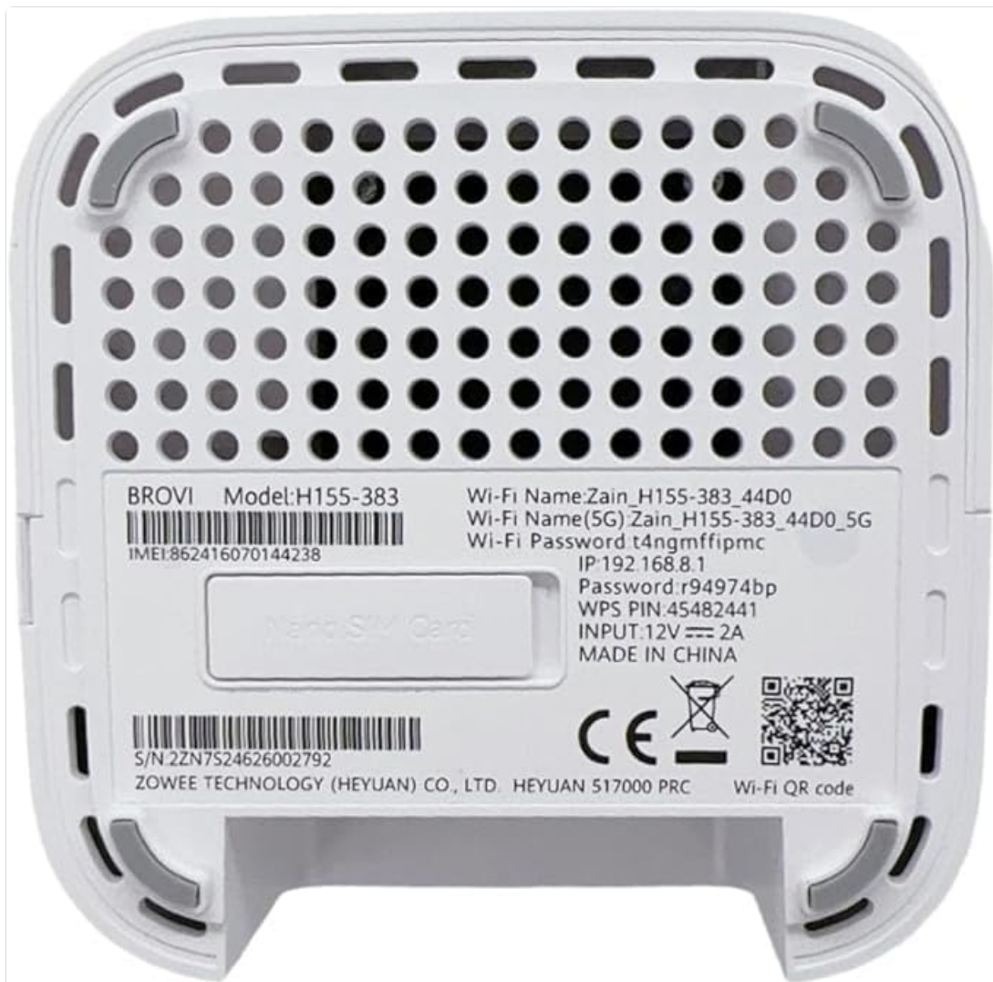
Figure 2: Router's bottom label, displaying essential network information such as default Wi-Fi SSIDs and password.
