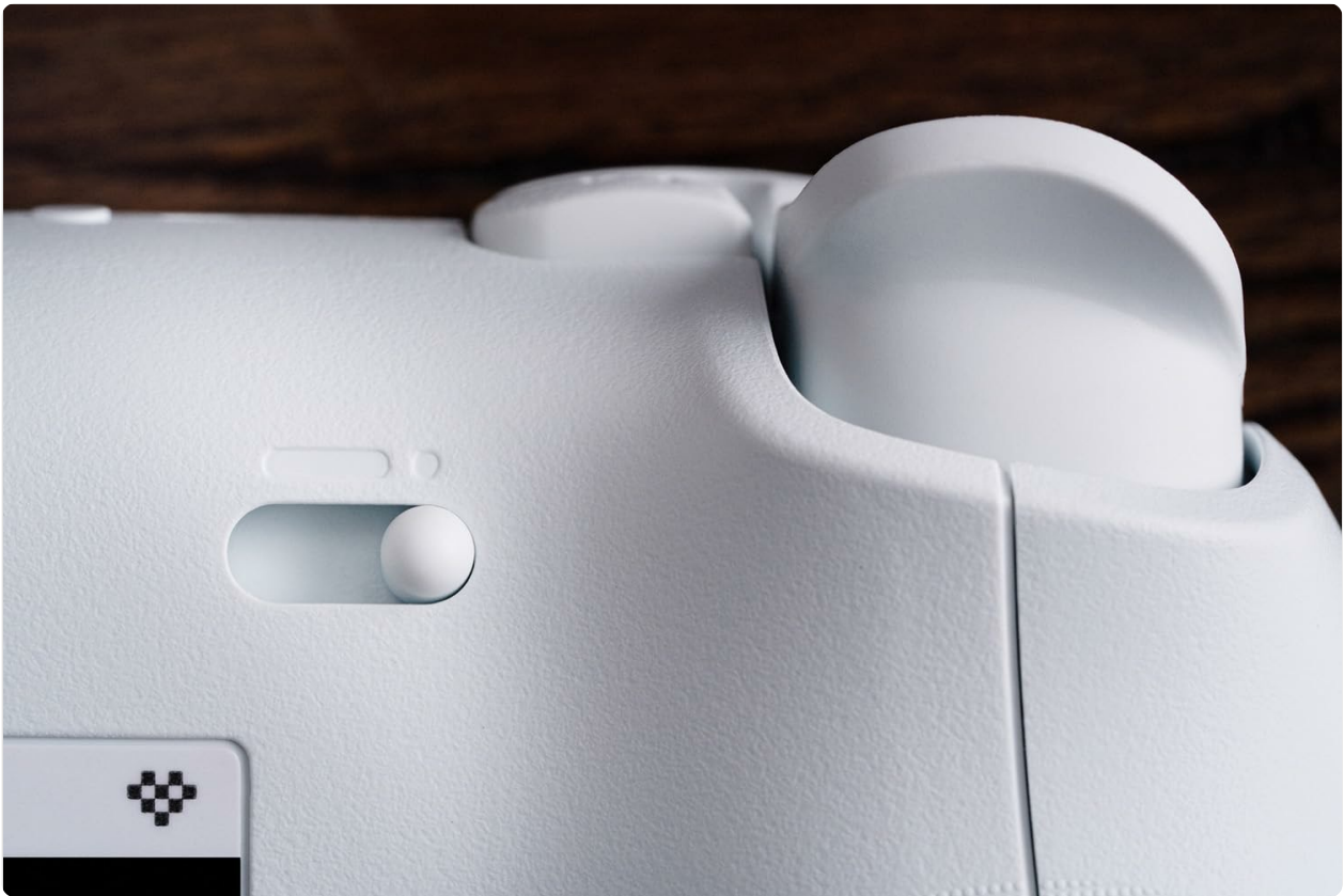
Image: A close-up of the physical switch on the controller's underside, used to change between Hall Effect and Tactile trigger modes.
