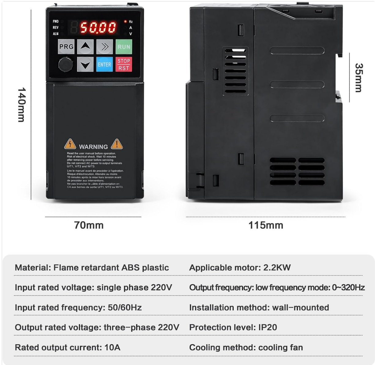
Figure 4.1: Physical dimensions of the DEWIN VFD, indicating its compact size for installation.
