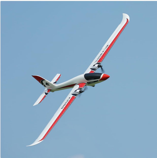
Figure 8.2: Underside view showing the twin power systems for enhanced thrust.
