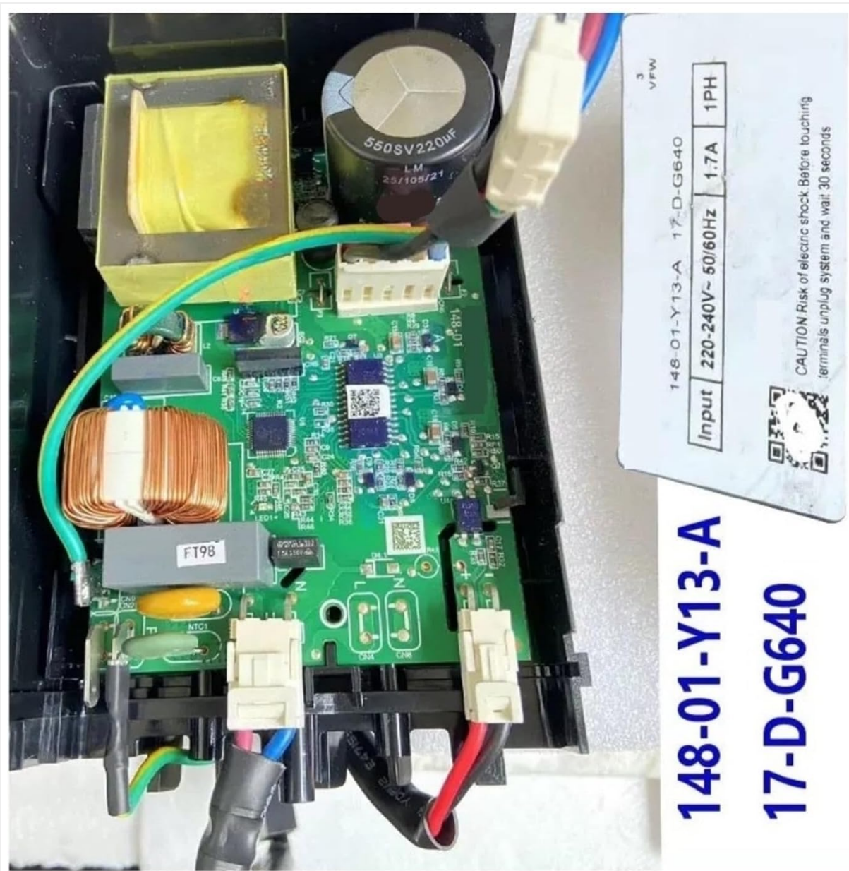
Image Description: A detailed view of the WWEIFUS Refrigerator Control Board, highlighting the various connection points for wiring harnesses. The board is mounted within a black plastic housing, and a label with model numbers and input specifications is partially visible.
