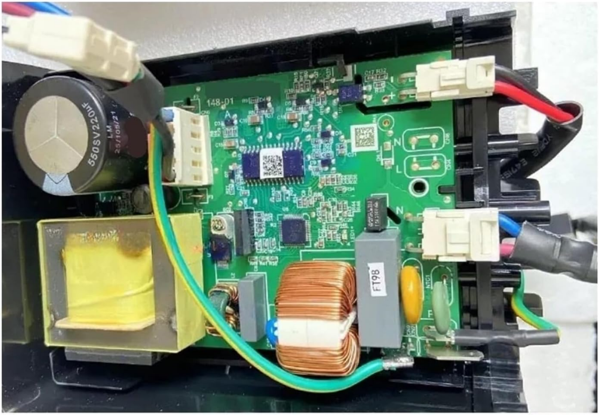
Image Description: An overhead view of the WWEIFUS Refrigerator Control Board, showing the layout of components and the main power input and output connections. The board is green, with a large capacitor and a copper coil transformer visible.
