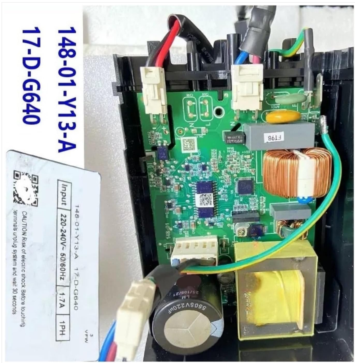
Image Description: The WEIFUS Refrigerator Control Board, showing the input specifications label clearly. The label indicates "148-01-Y13-A 17-D-G640" and "Input 220-240V~ 50/60Hz 1.7A 1PH". A warning about electric shock is also visible.
