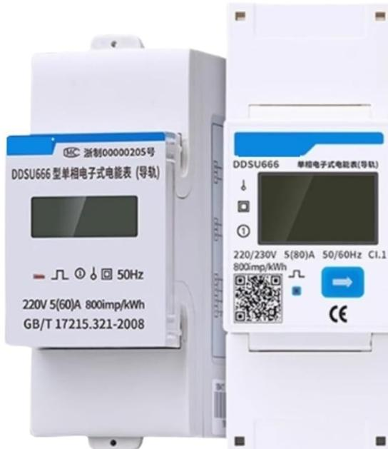
This image displays two SOBOUR DDSU666 single-phase electronic energy meters designed for DIN rail mounting. Both meters feature an LCD screen for displaying energy consumption data. The left meter shows specifications including 220V 5(60)A, 800imp/kWh, and compliance with GB/T 17215.321-2008. The right meter indicates 220/230V 5(80)A 50/60Hz, C1.1, 800imp/kWh, and a CE mark, along with an RS485 symbol, suggesting communication capabilities.
