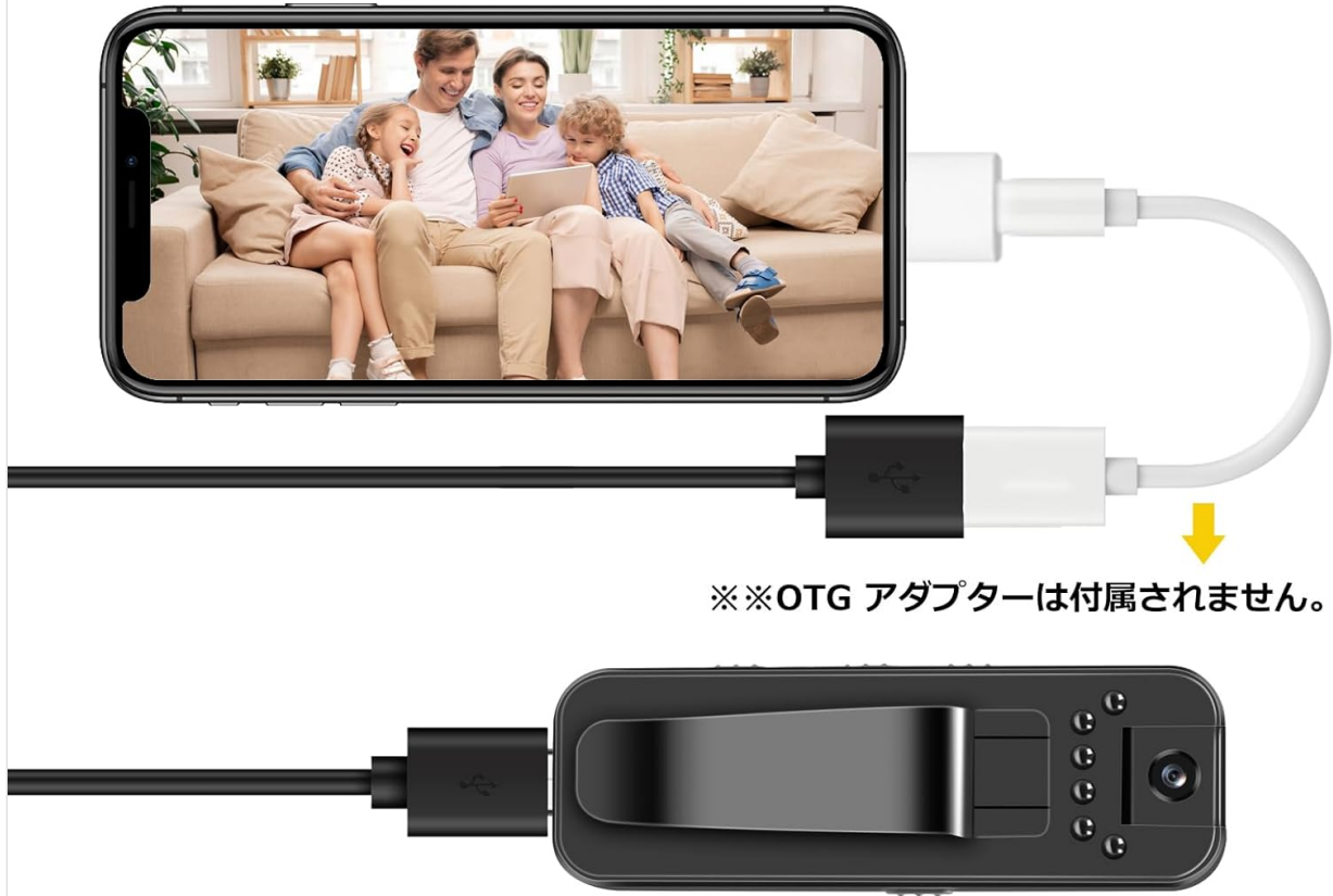
Figure 5.5: OTG Functionality. This image demonstrates connecting the camera to an Android smartphone via a USB cable and an OTG adapter, allowing direct viewing of video files on the phone.
