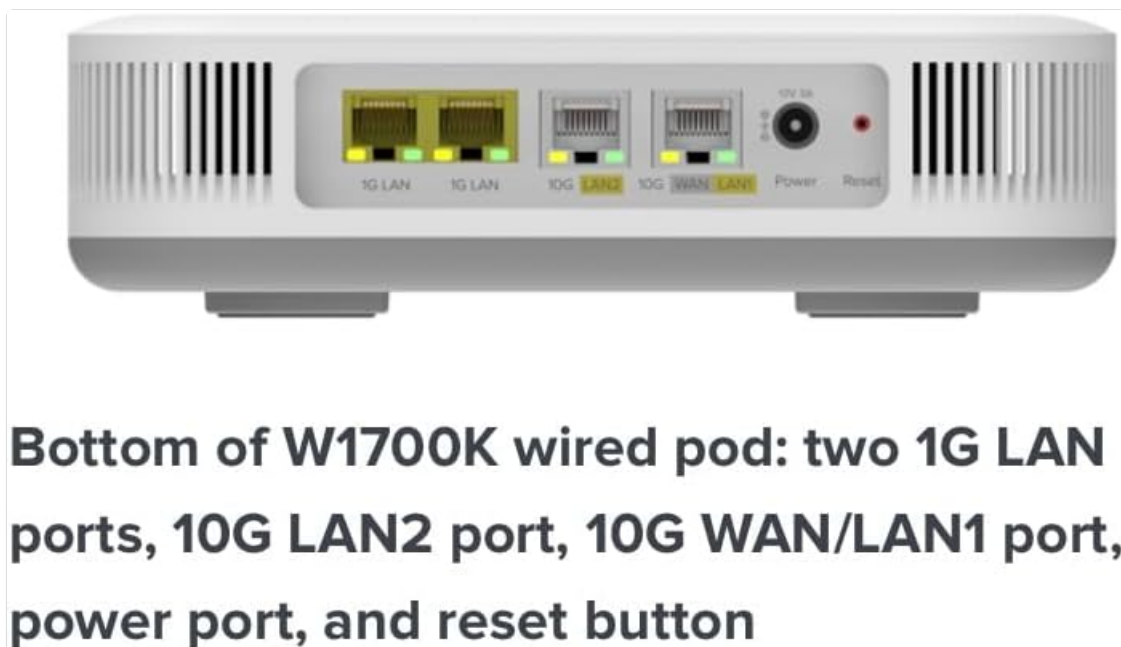
Figure 4: Detailed view of the W1700K Wired POD's ports.
