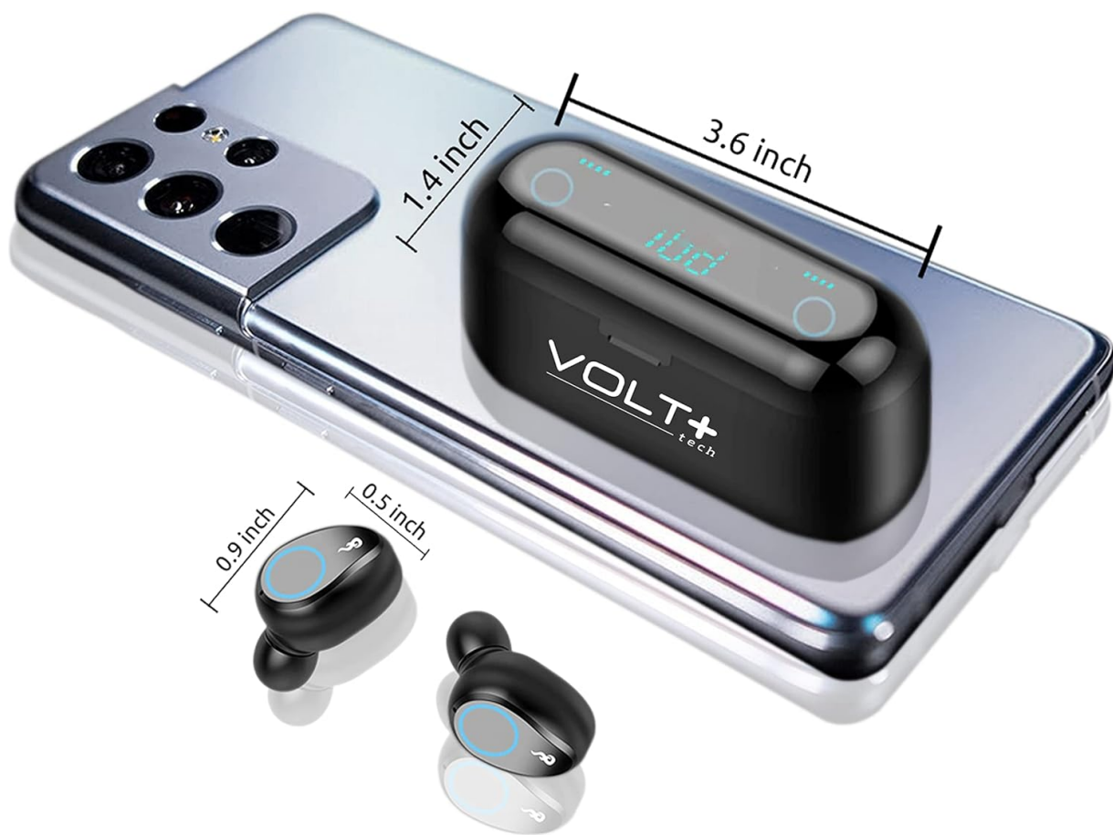
Image 8.1: Physical dimensions of the earbuds and charging case.
