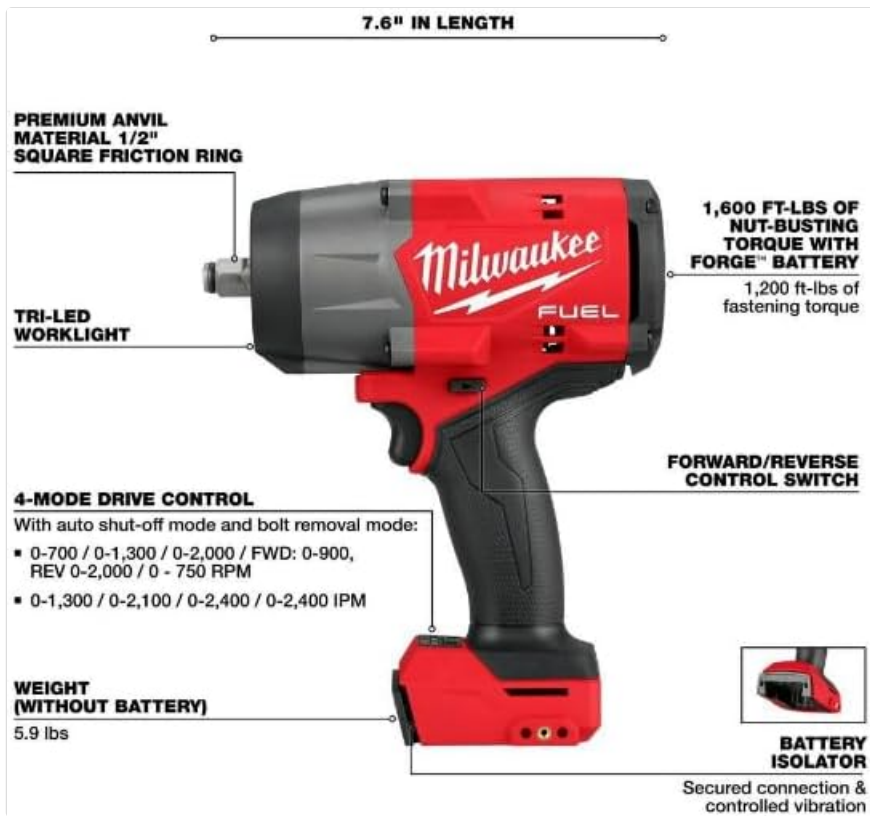
Image Description: A detailed diagram of the Milwaukee M18 FUEL Impact Wrench, pointing out key features such as the 1/2" square friction ring anvil, Tri-LED worklight, 4-Mode DRIVE CONTROL, forward/reverse control switch, battery isolator, and weight. This image helps users identify different parts of the tool.
