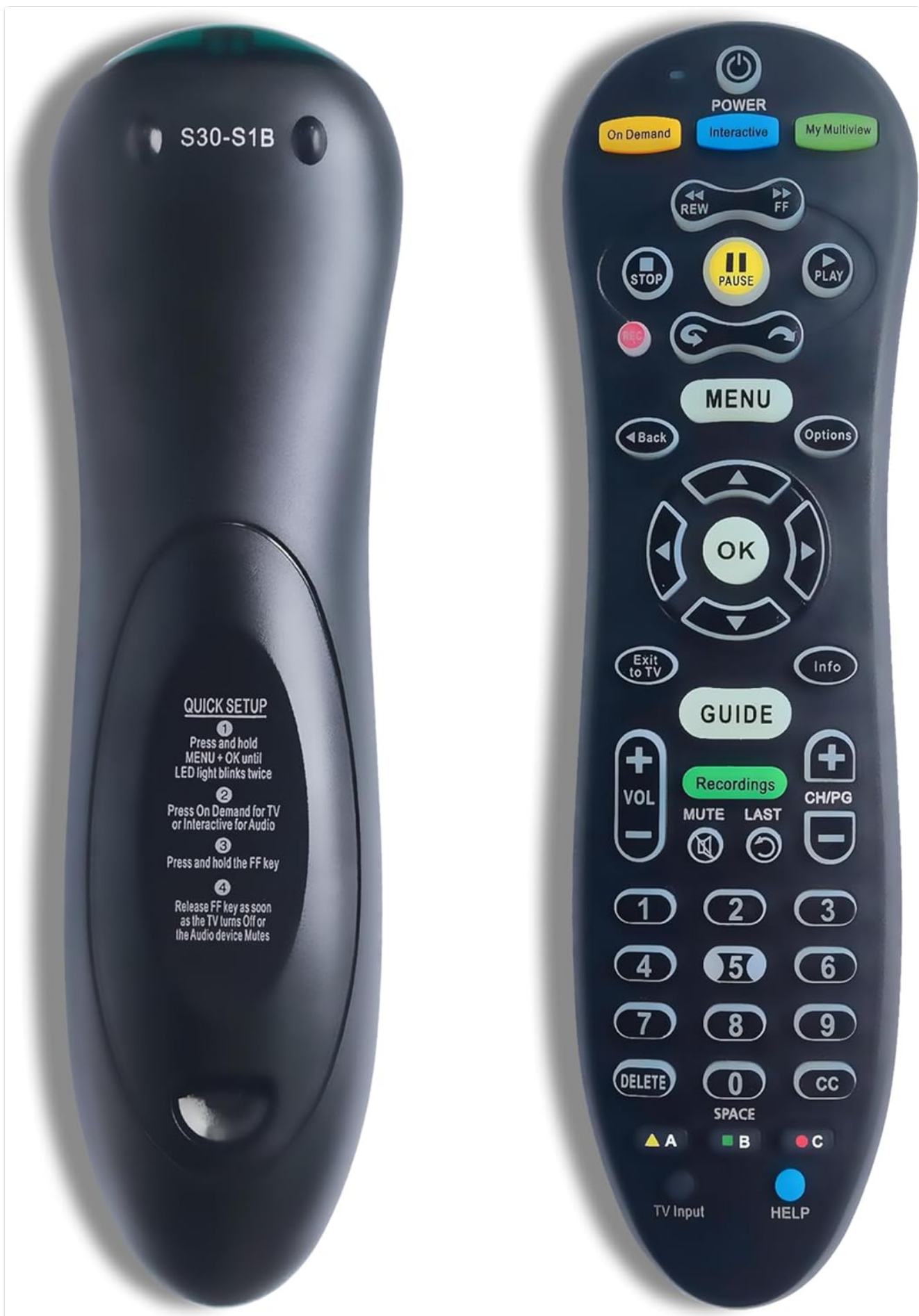
Image: Front and back view of the Generic S30 Universal Remote Control. The front displays the array of control buttons including power, channel, volume, navigation, and number keys. The back panel features a label with the model number S30-S1B and a "QUICK SETUP" guide with four steps for pairing.
