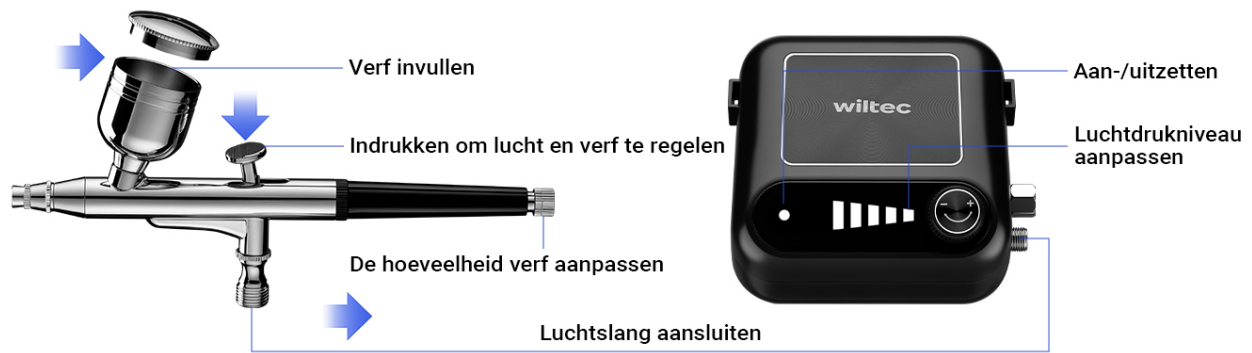
Figure 5.1: Simple operation and connection diagram.
