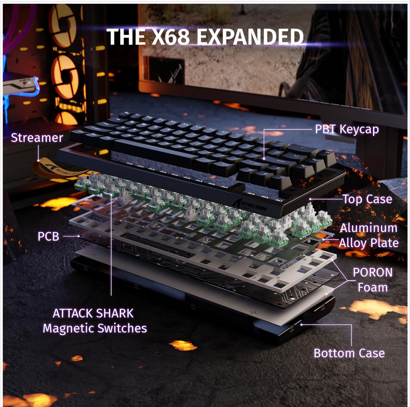
Image: An exploded diagram of the X68 HE keyboard, showing its internal components including PBT keycaps, top case, aluminum alloy plate, PORON foam, PCB, and ATTACK SHARK magnetic switches.
