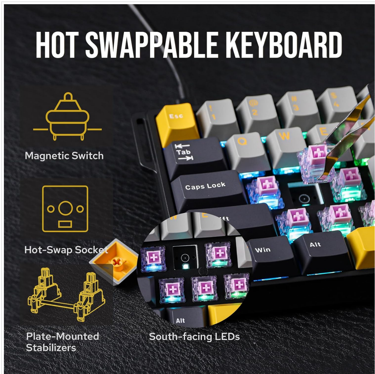
Image 5.4: Hot-swappable design with magnetic switches and south-facing LEDs.
