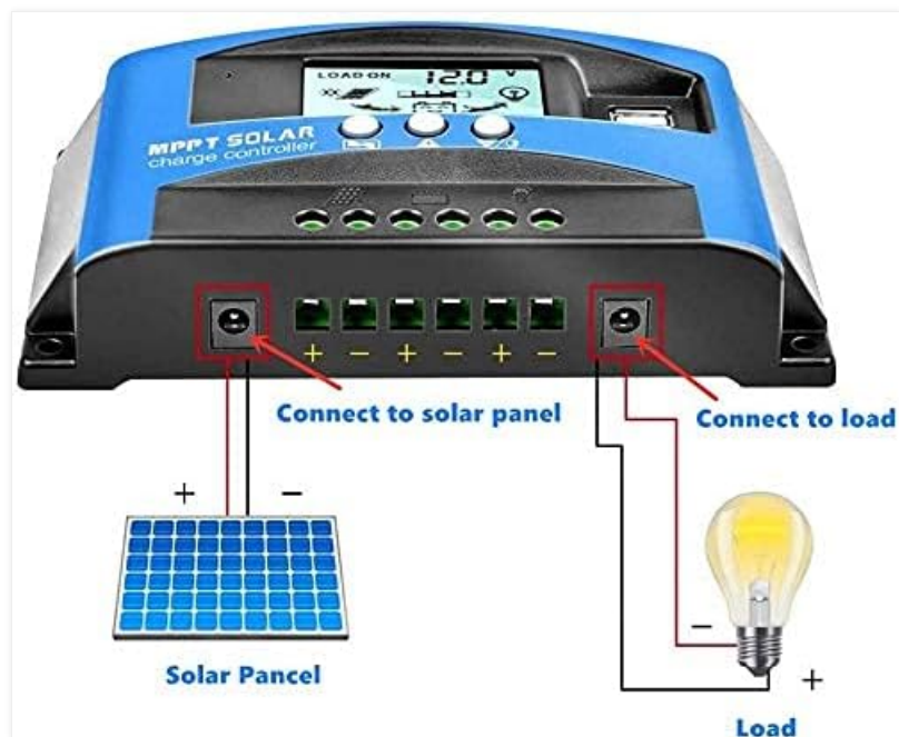
Figure 3: Basic wiring diagram showing connections from a solar panel to the controller and from the controller to a DC load. Note the positive (+) and negative (-) terminals.
