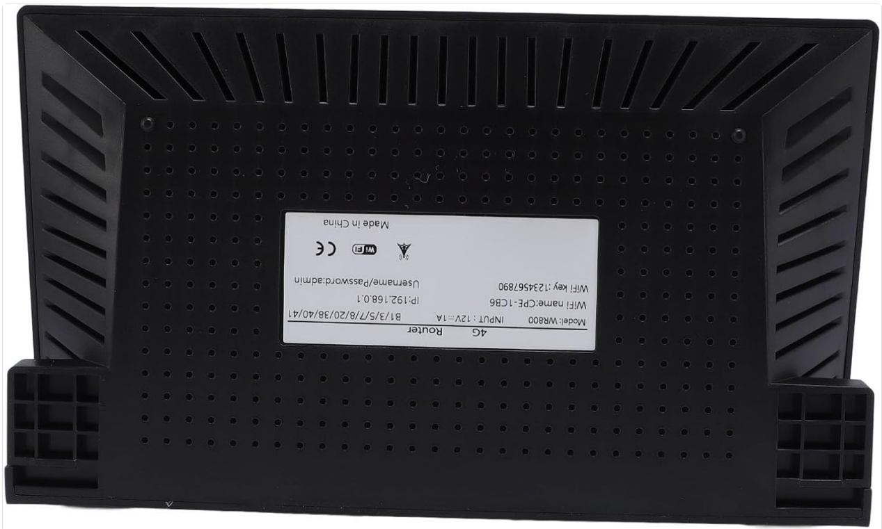
Image: The bottom label of the Bewinner WR800 router, displaying essential information such as the model number, default WiFi name, WiFi key, and router IP address (192.168.0.1).
