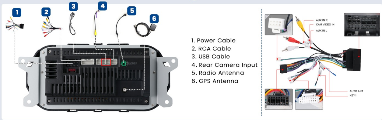
Figure 3.1: Rear view of the autoradio showing numbered wiring ports and a detailed connection diagram for the main harness.
