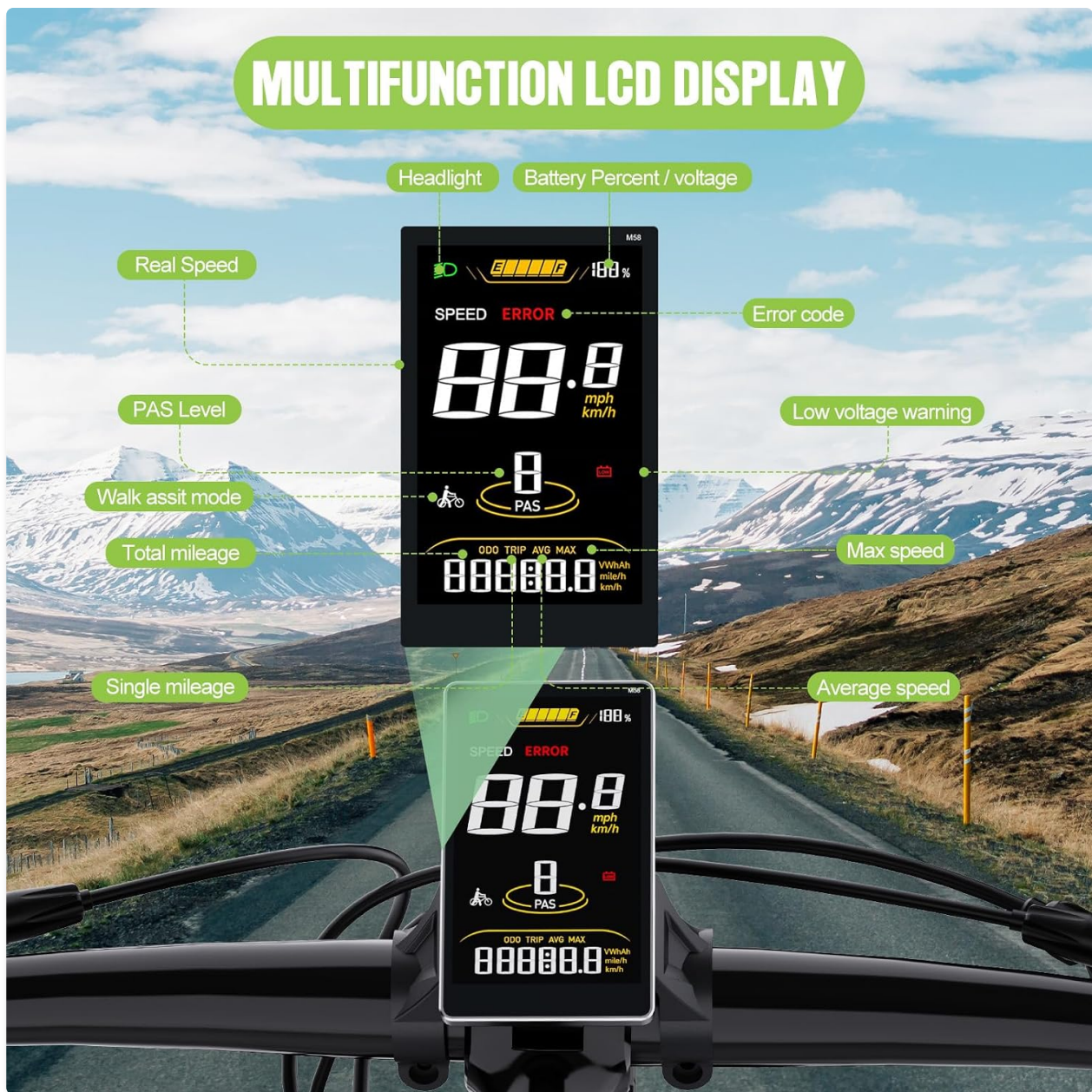
Figure 5: Annotated diagram of the SW2M58 display screen, highlighting all key data points and indicators.
