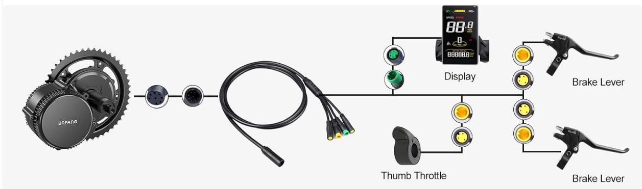
Figure 3: Detailed wiring diagram for the 5-pin connectors and a system overview showing how the display integrates with other ebike components.
