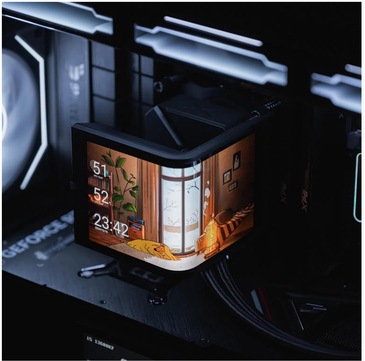
Figure 7: The AIO cooler's screen displaying the "Waterfall Mode" animation, optimized for vertical screen orientation and showing system statistics.
