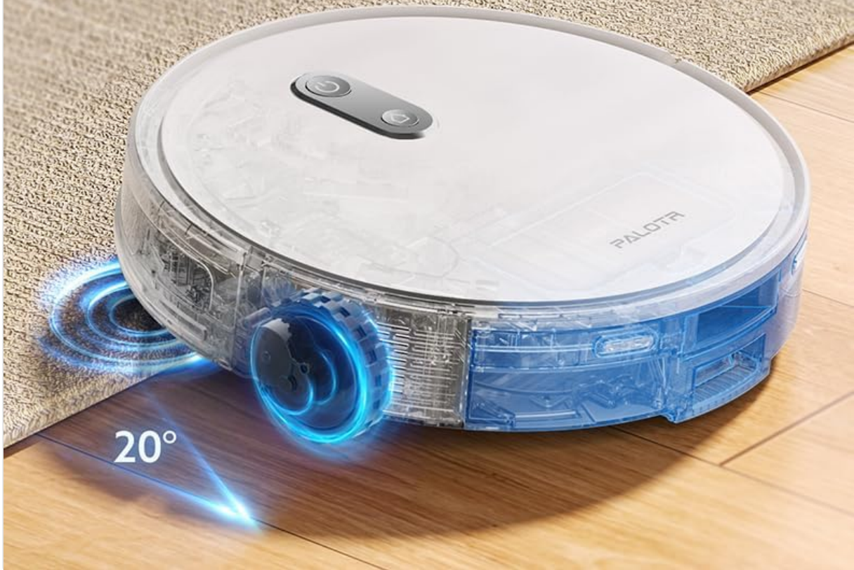
Figure 4.4: The robot demonstrating its ability to climb over obstacles, such as carpet edges, up to a 20-degree incline.
