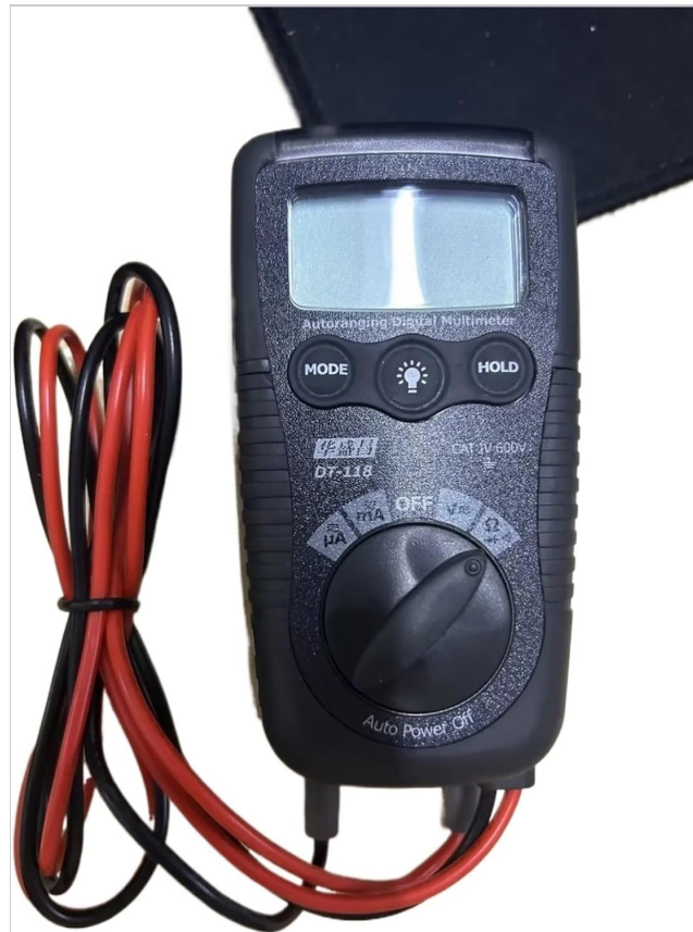
Figure 3.1: The DT-118 multimeter with its red and black test leads properly connected to the input jacks, ready for use.
