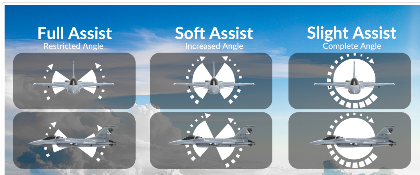
Figure 3: Visual representation of the 3-Level Flight Control modes.
