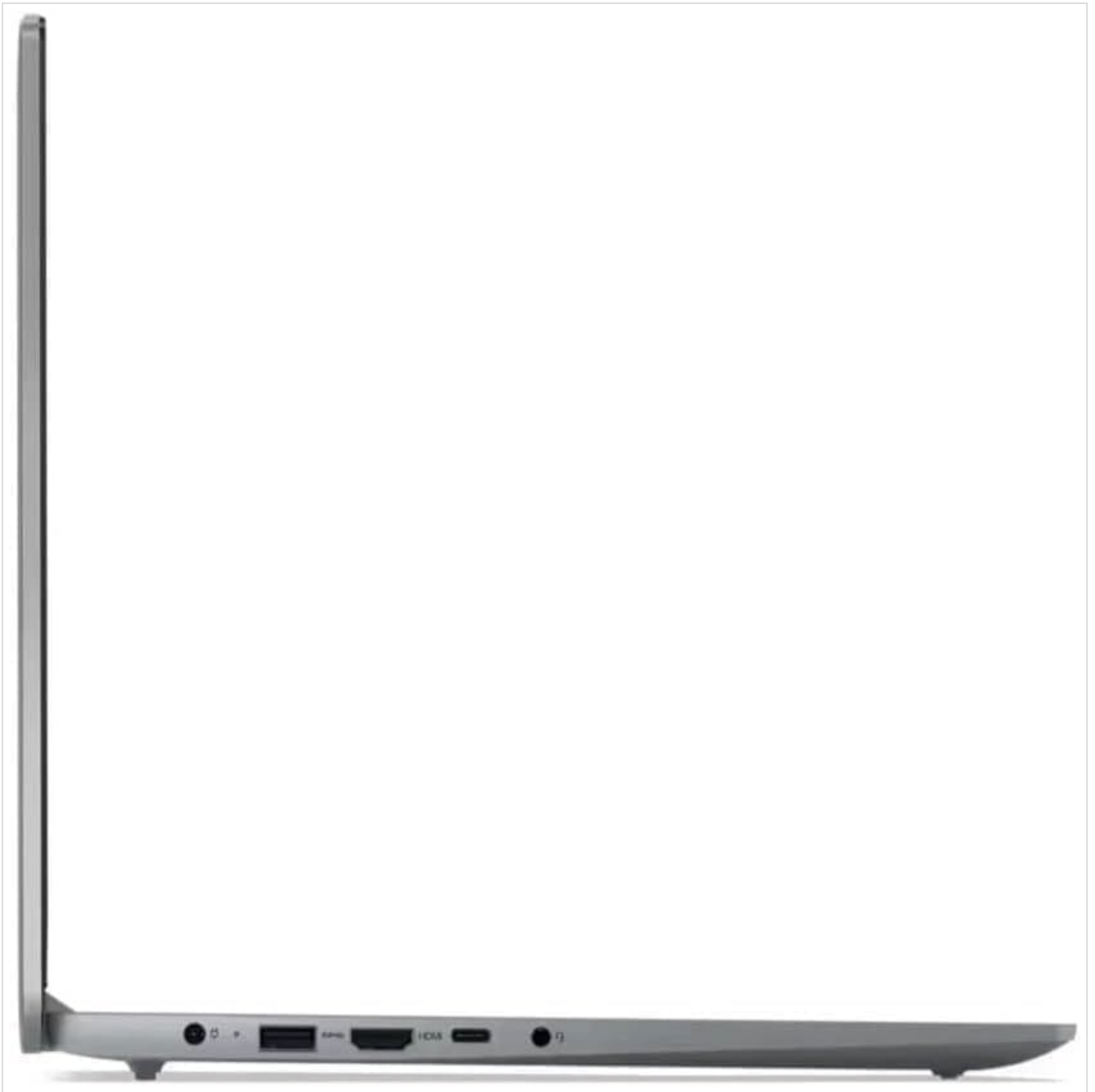
Image: Left side of the laptop, showing the power input, USB ports, HDMI port, and USB-C port.
