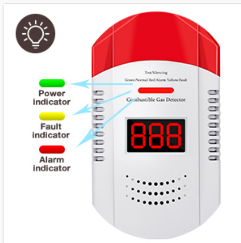
Figure 5.1: Indicator lights and their meanings.
