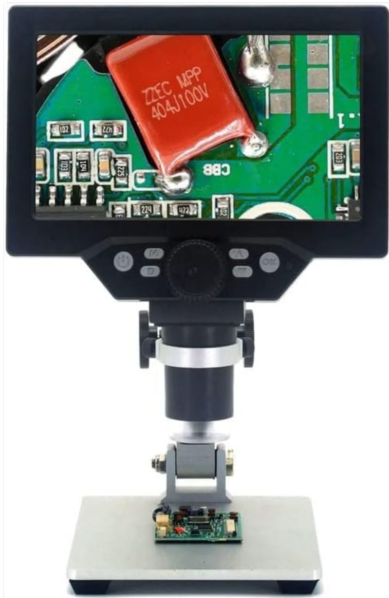
Figure 4.3: The G1200 features a 7-inch display for enhanced viewing clarity.
