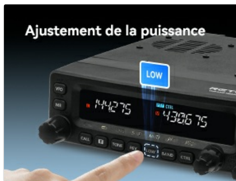
Image 5.2: The 'LOW' button for adjusting the radio's power output.
