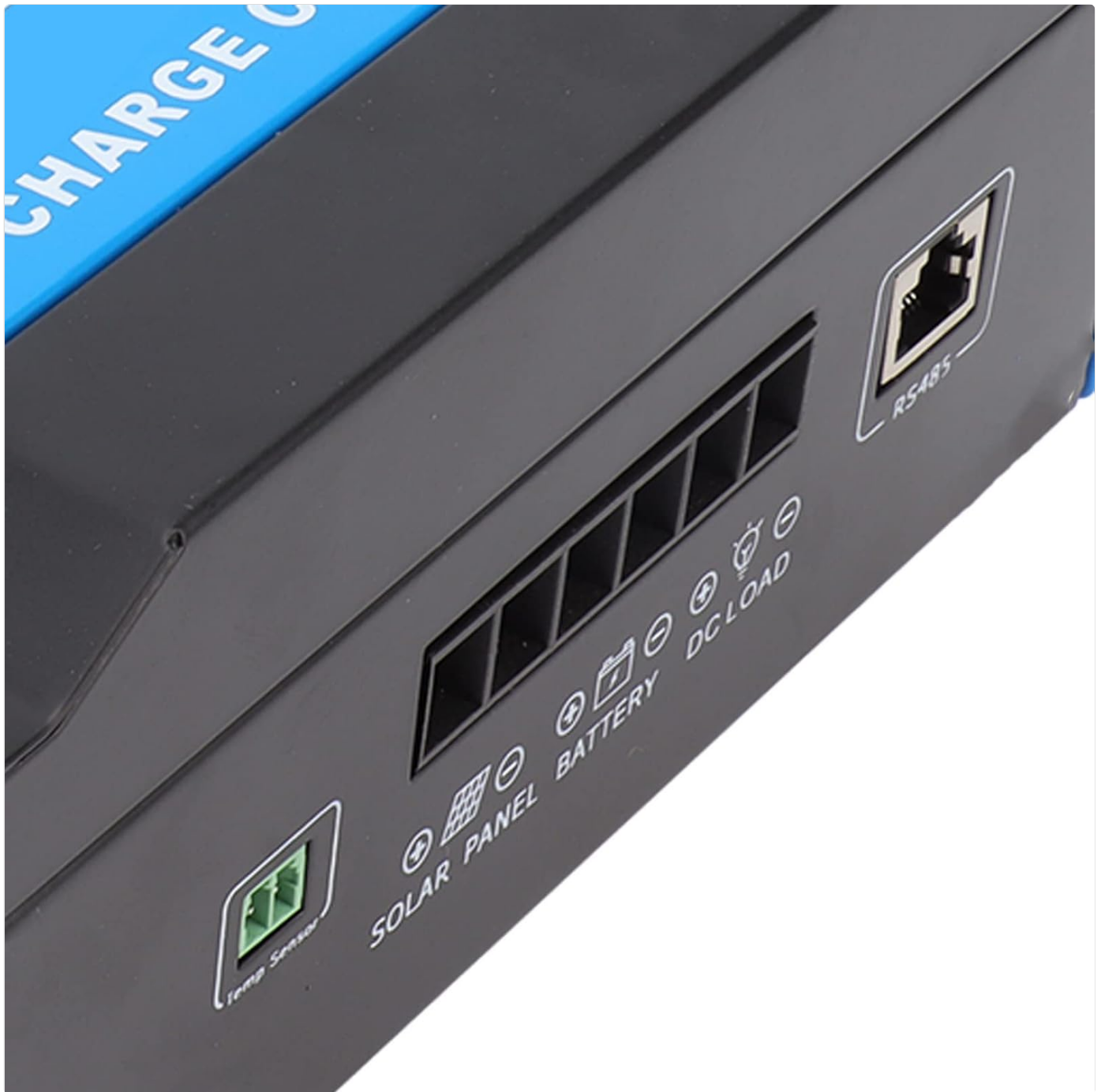
Figure 5.2: Detailed view of the connection terminals located at the bottom of the controller.
