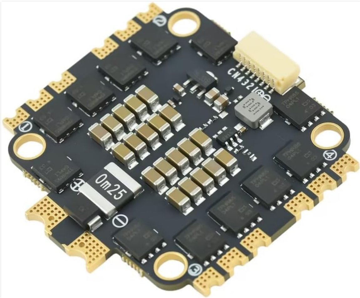
Figure 4.4: Angled View 1. A perspective view of the ESC, illustrating its compact form factor.
