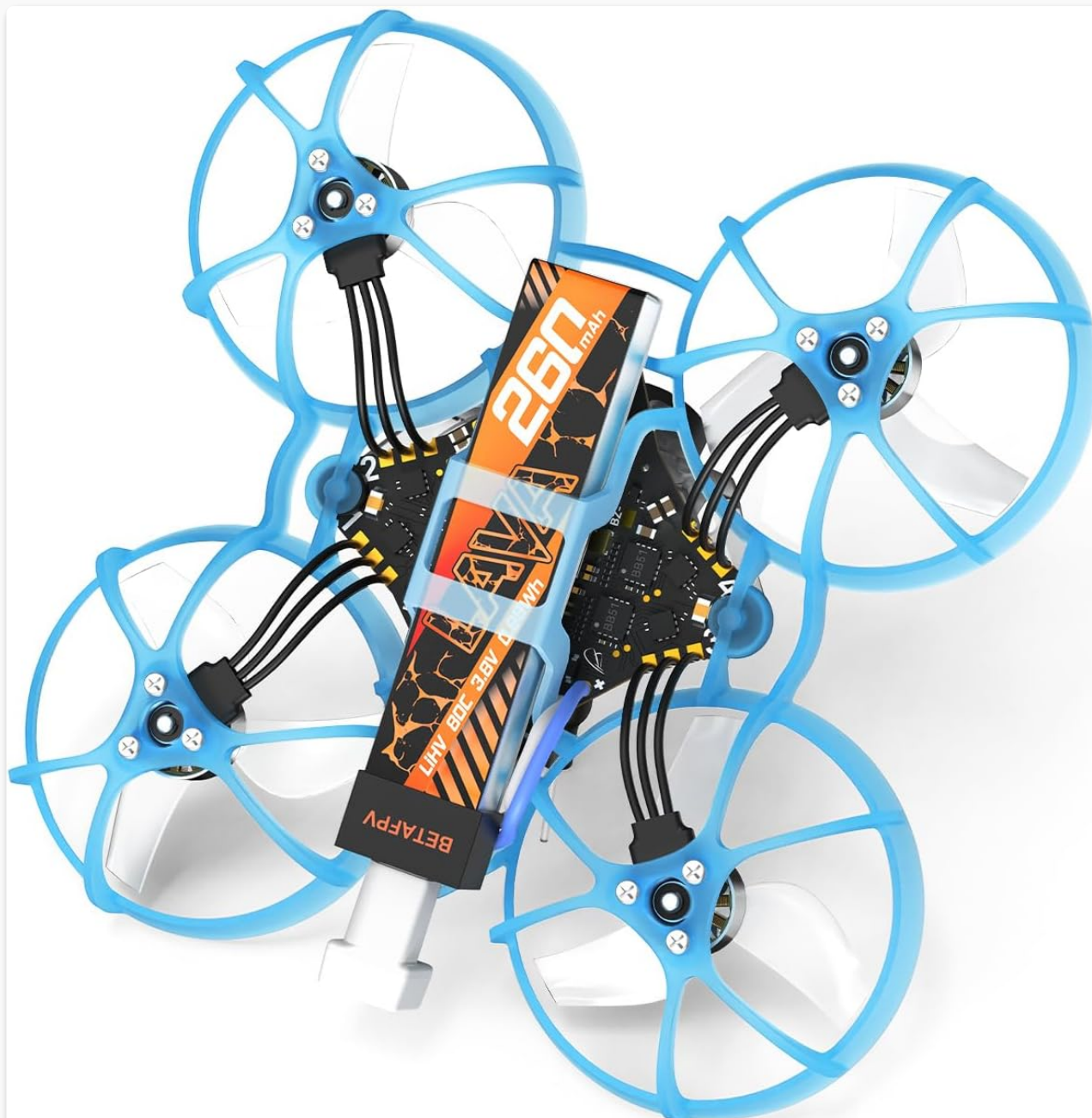
Image 6: Illustration of how to properly install the 1S LiPo battery into the Air65 quadcopter.
