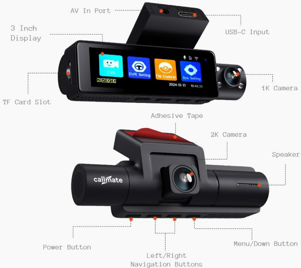
Figure 3.1: Front and rear view of the CALLMATE Roadventurer Dash Camera with key components labeled. These include the 3-inch IPS Display, TF Card Slot, AV In Port, USB-C Input, 1K Camera (interior), 2K Camera (front), Speaker, Power Button, Left/Right Navigation Buttons, Menu/Down Button, and Adhesive Tape for mounting.
