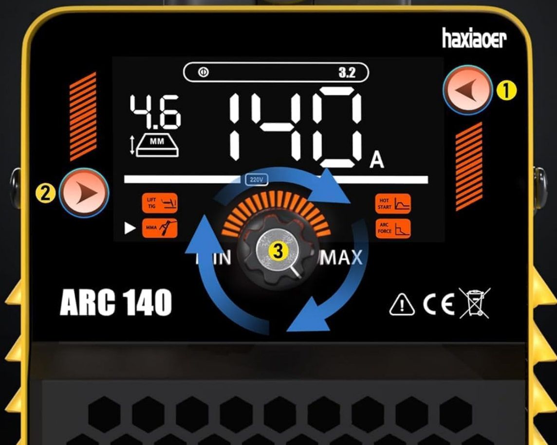
Image: A detailed view of the welder's control panel, highlighting the 3-key button operation for VRD, Welding Mode, and Parameter Knob, simplifying adjustments.
