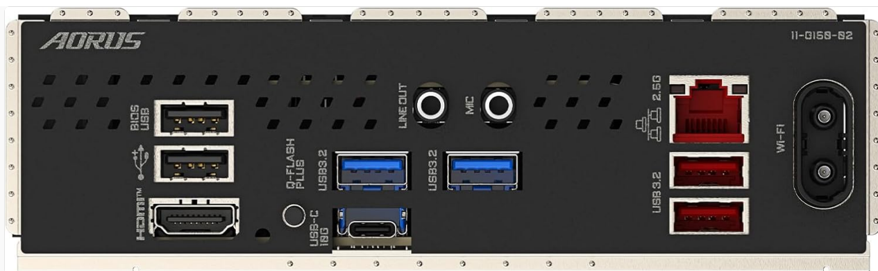
Image: Rear I/O panel of the GIGABYTE B850I AORUS PRO Motherboard, showing various ports including USB, HDMI, LAN, and audio jacks.
