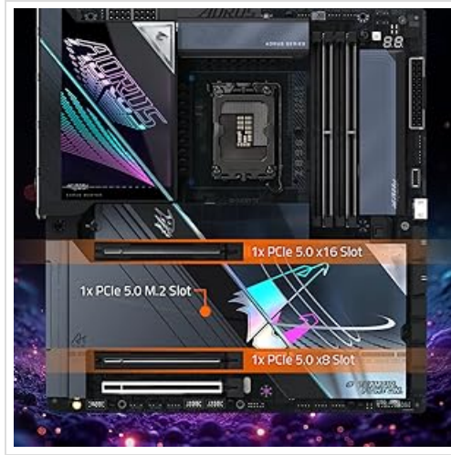
Figure 6: PCIe 5.0 slots for graphics cards and expansion.
