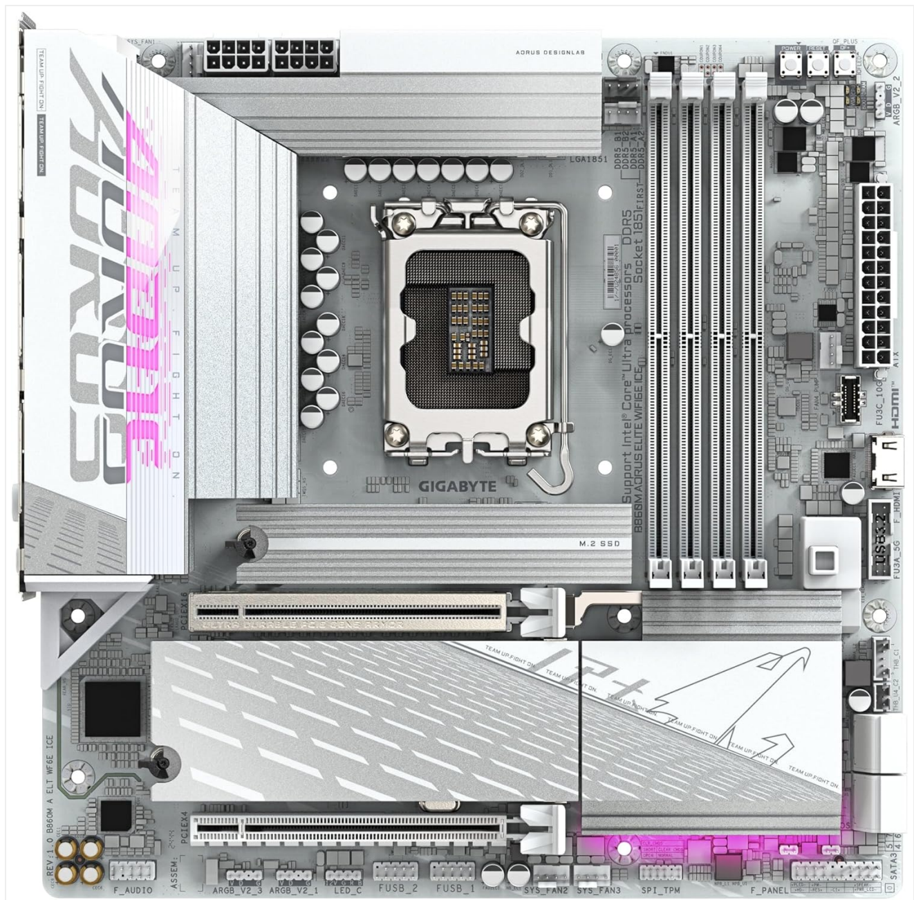
Image 3.1: Top-down view of the motherboard, highlighting the CPU socket, DIMM slots, and M.2 slots.
