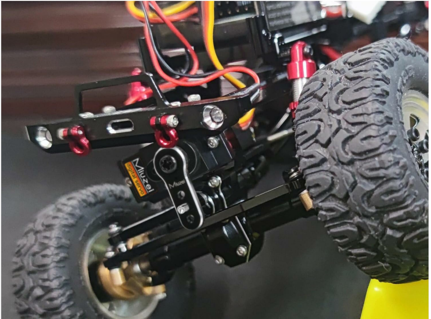
Image: The servo in an RC crawler, illustrating its precise angle control during operation.
