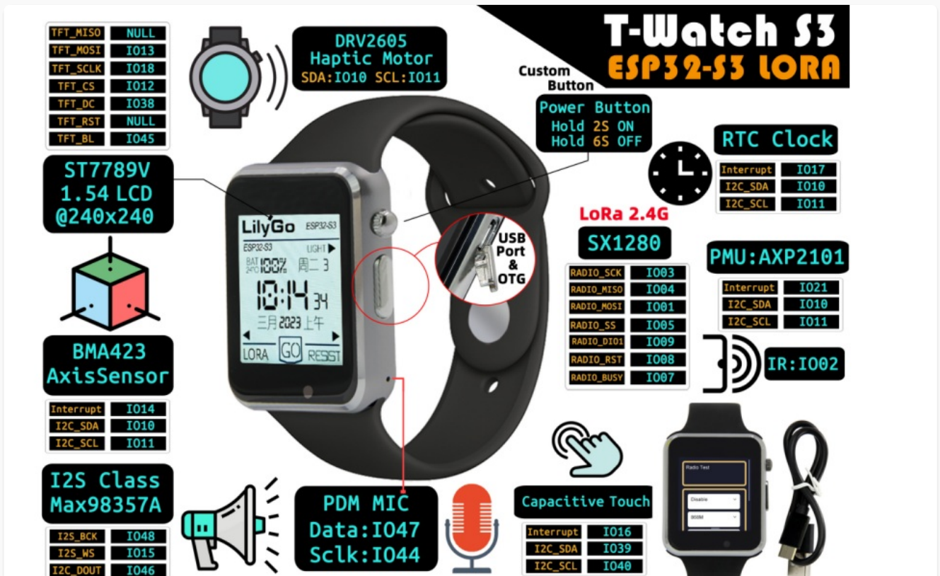
Figure 2.3.5: Detailed internal component layout and pinout diagram of the T-Watch-S3.
