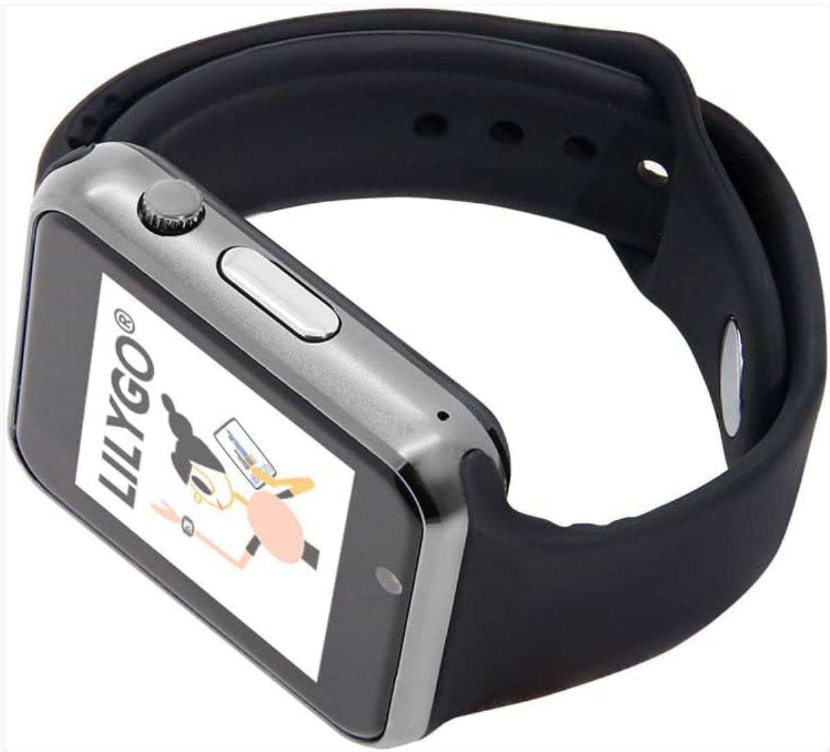
Figure 2.3.2: Side view of the T-Watch-S3, highlighting the crown and side button.
