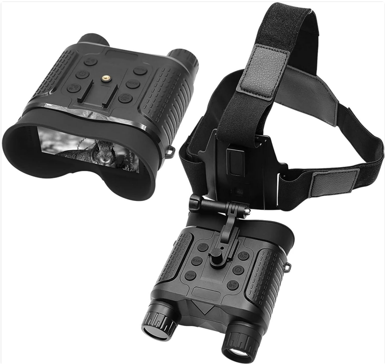
Figure 6.2: The NV8160 binoculars with the head strap, showing the display screen with a black and white image of a squirrel, illustrating one of the available color effects for night vision.
