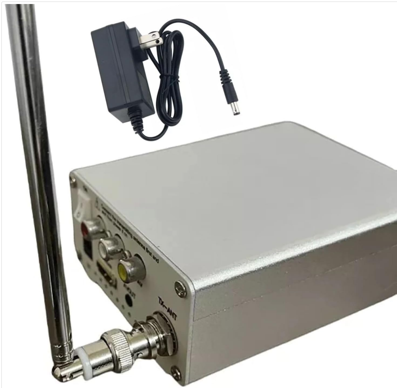
Image: The telescopic antenna connected to the TX-ANT port on the rear of the device.
