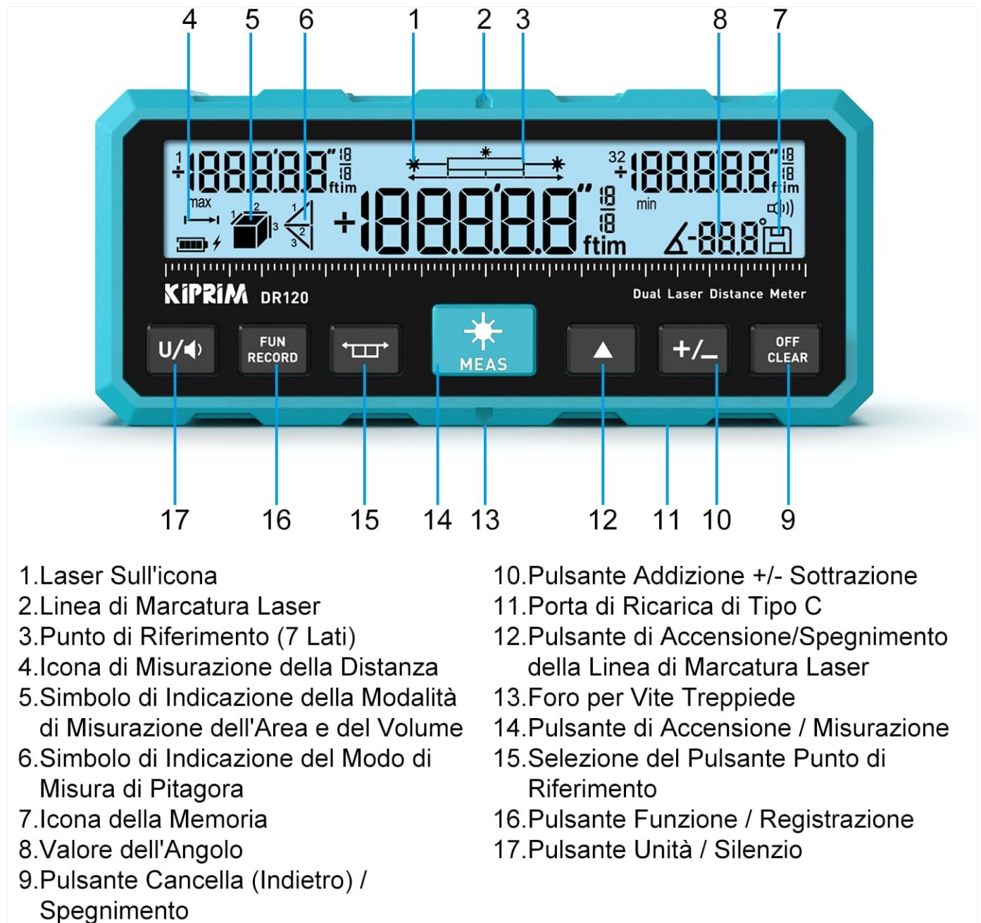
Figure 2: KIPRIM DR120 Laser Distance Meter Parts Diagram.
