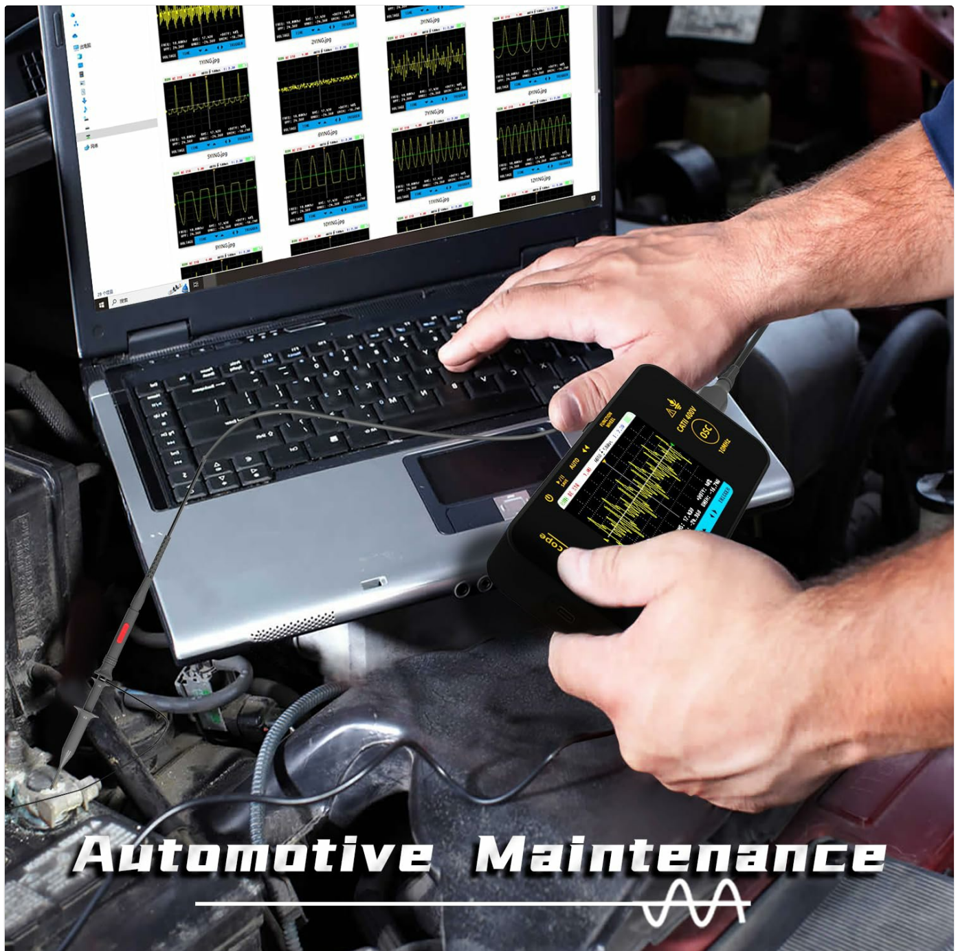
Figure 7.1: The BSIDE OT3 being used for automotive maintenance, demonstrating its application in vehicle diagnostics and its ability to connect to a PC for data review.
