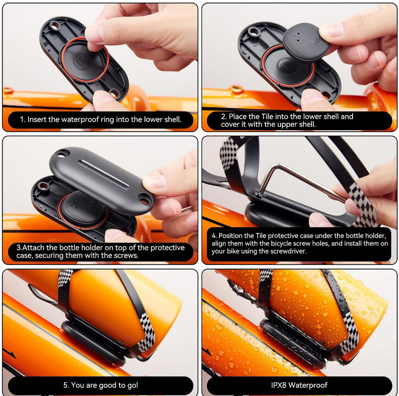
Image: Visual guide for inserting the waterproof ring into the lower shell.
